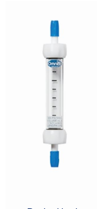
Packed bed Heterogeneous catalysis, scavengers
